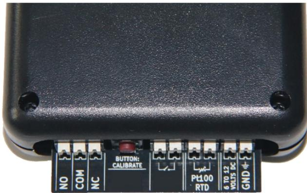
**LD-215 Liquid Nitrogen Level Detector/Alarm Connections**
